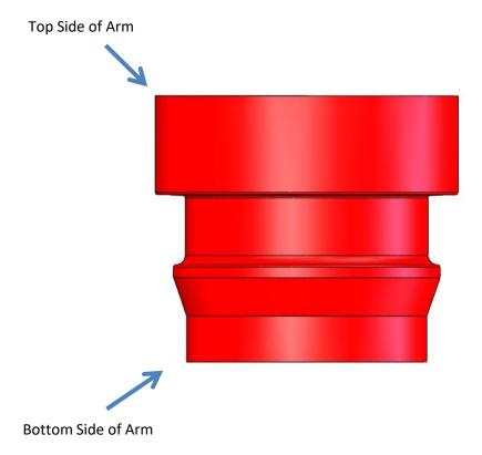
No grease is required. Use tyre soap or washing up liquid to aid with fitment.
